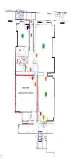
Fire Estinguisher Co2 Fire Estinguisher Foam Fire Estinguisher Water Smoke Dector Emergercy Light Break Glass Call Point Fire Alarm Sounder Fire Alarm Panel Stairs Access and Egress Area of Performance
